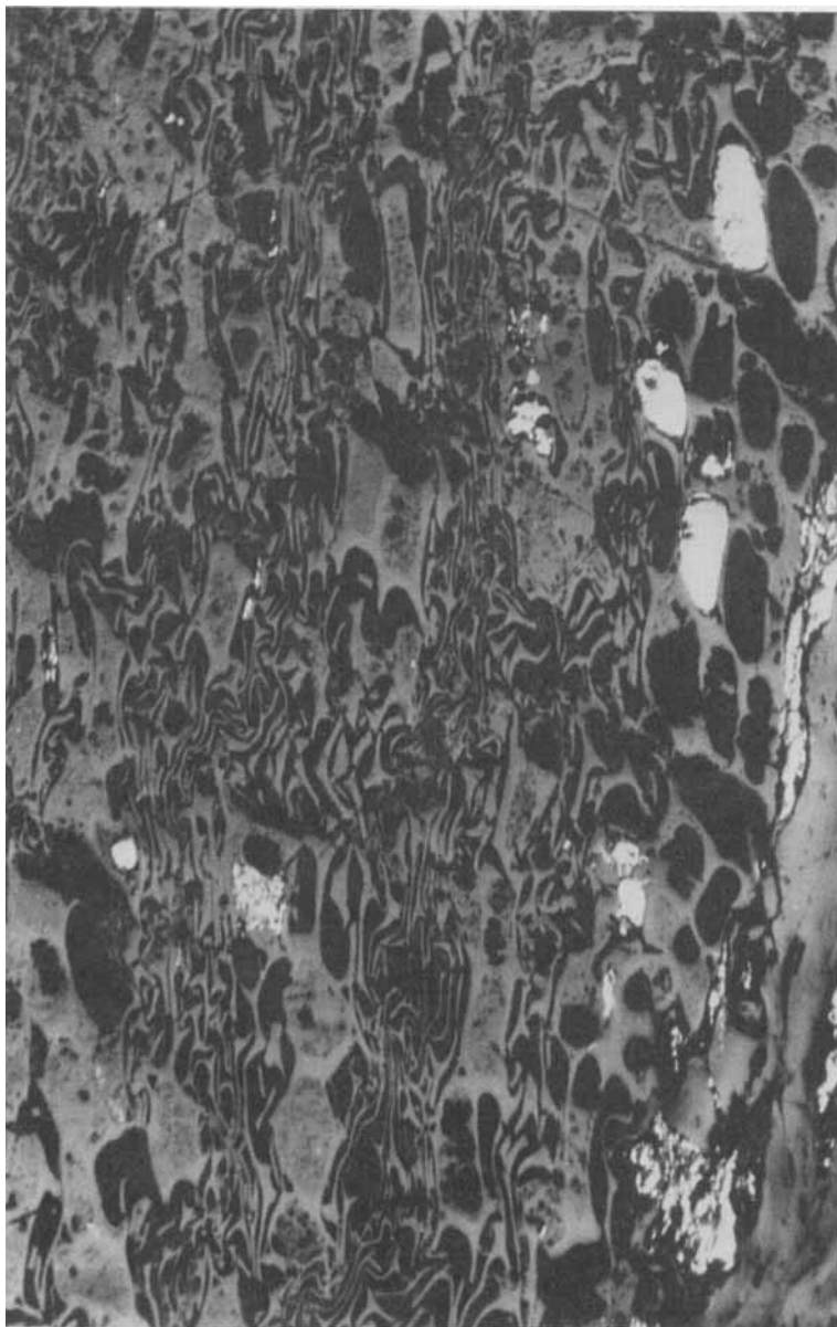
FIGURE 4. Pyrite occurring within cell lumens in fusinite in the same coal as that shown in Figure 3. Reflected light, oil immersion, field width 0.5 mm.
