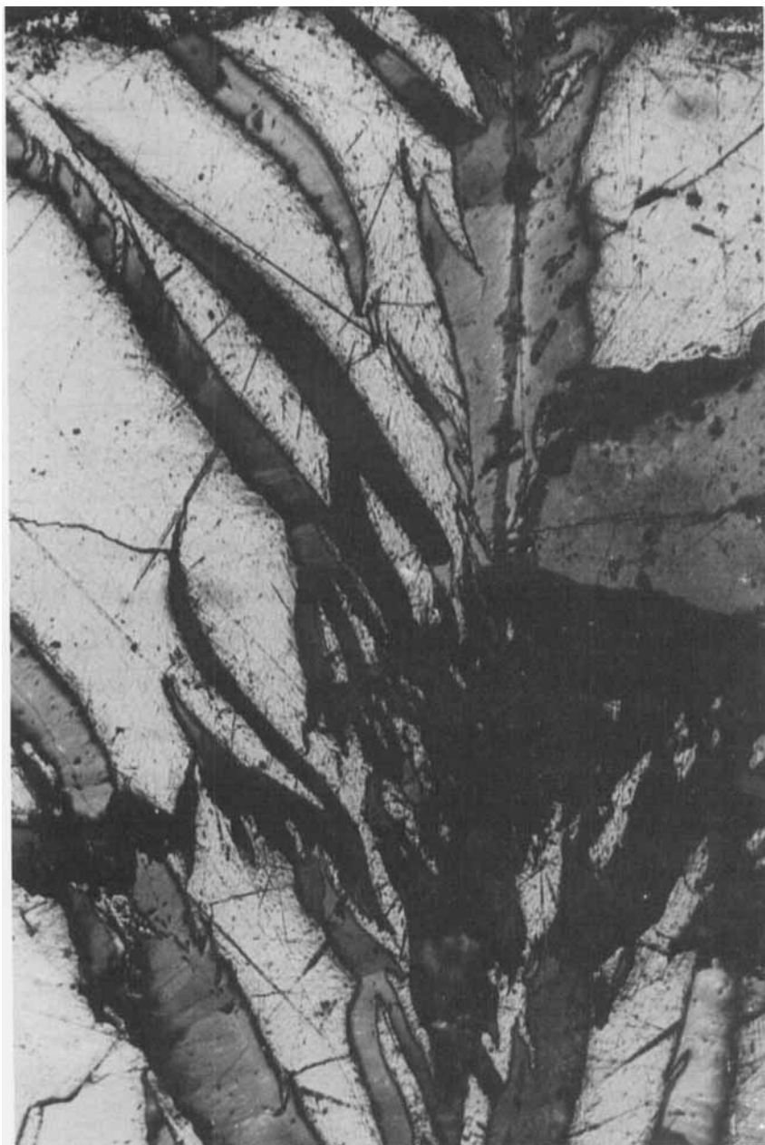
FIGURE 11. Calcite of epigenetic origin occurring as veins within vitrinite. Coal from Singleton Coal Measures, Goulburn Calley No. 1 borehold, N.S.W. Reflected light, oil immersion, field width 0.5 mm.
