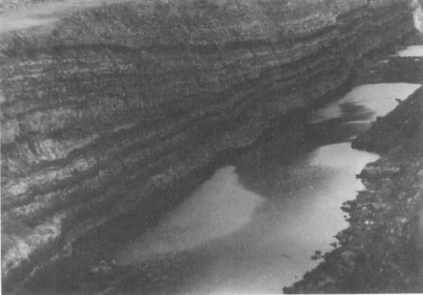
FIGURE 7. Overburden strata at the Costain Opencut, Liddell, N.S.W. Part of the seam (approx. 3 m) is exposed at the base of the high wall (40 m in height).
